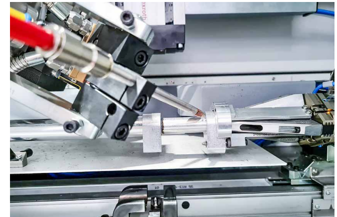
Laser welding with a cold wire system offers the highest precision.
